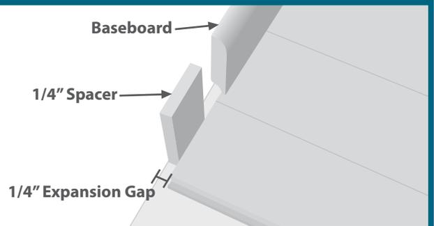
Leave at least 1/4" expansion spaces between flooring and ALL vertical objects (walls, cabinets, pipes, etc.) Large flooring runs may require additional expansion space. Undercut door jambs and casings to provide adequate expansion space. Cali Bamboo® does not recommend screwing or nailing cabinetry or other permanent fixtures to the flooring.
